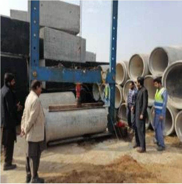
Picture 63: 3-Edge Bearing Testing for RCC Pipe
